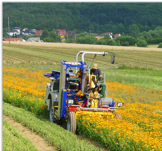
The self-developed flower harvesting machine removes the calendula blossoms cleanly from the crop. (Photo: Krebsbachhof)
